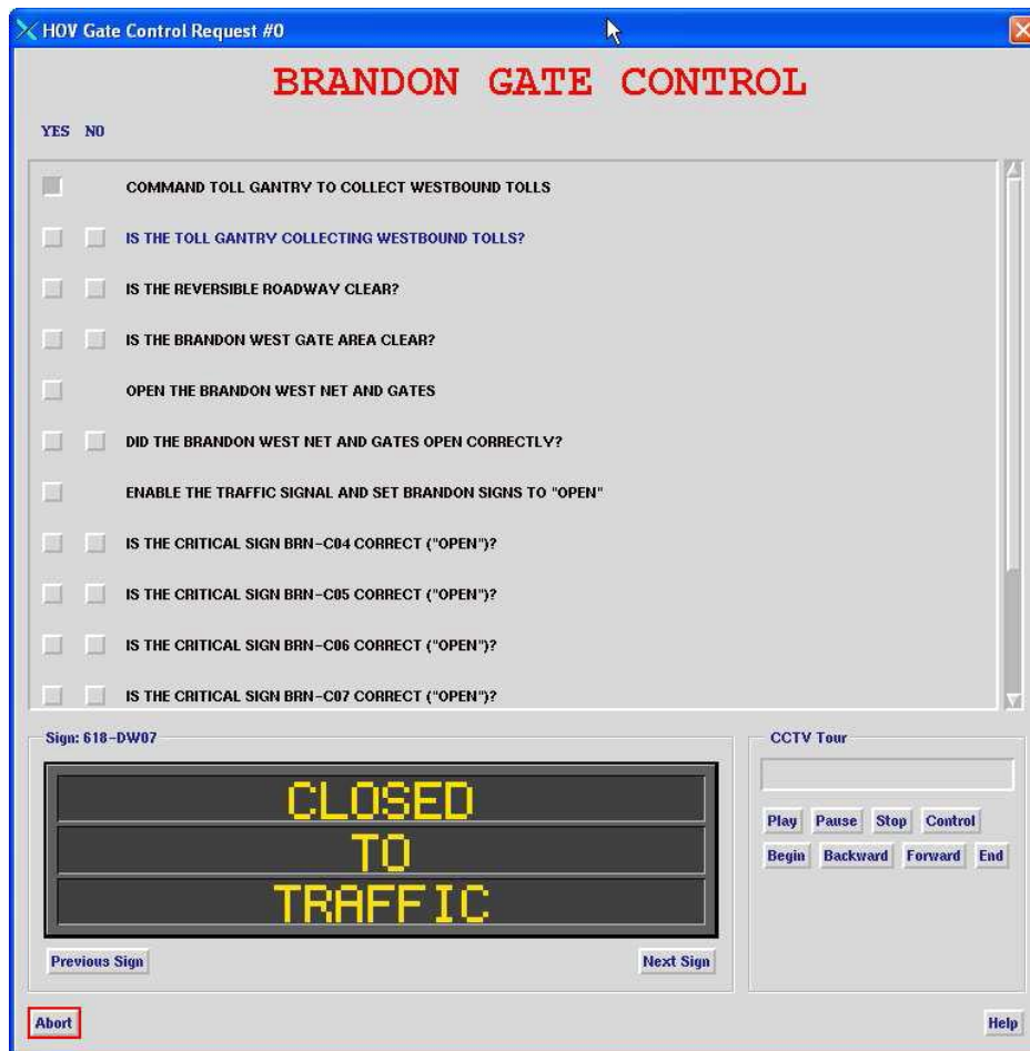
Figure 1-3: ORT LC “Switch” command via DynGate™ Checklist
